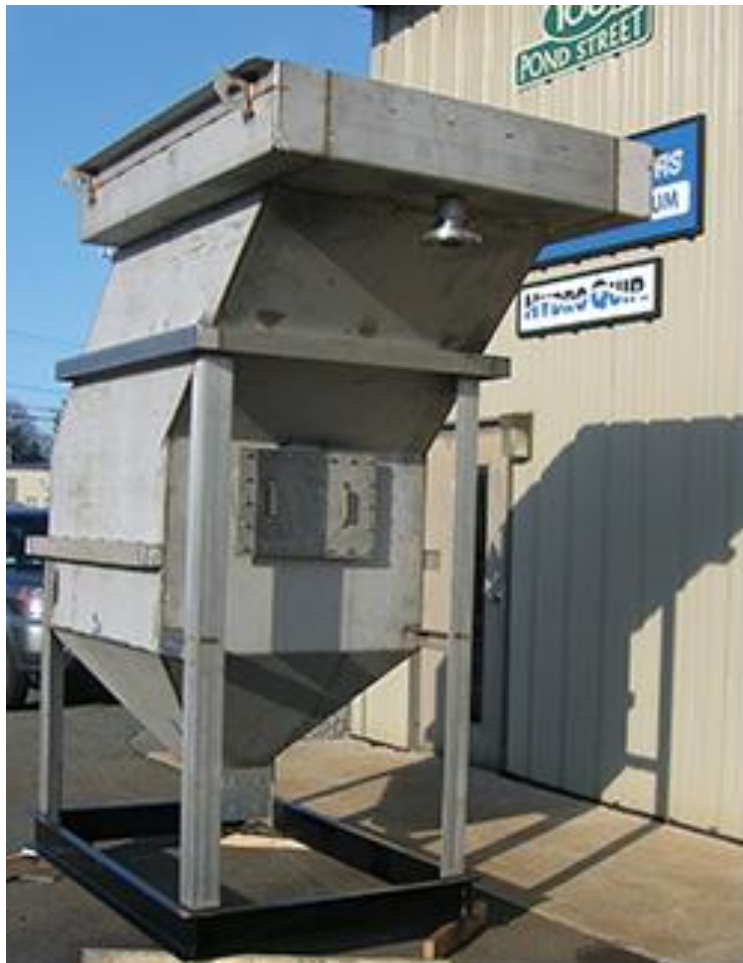
Figure 30: Inclined plate clarifier
